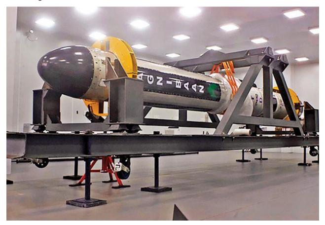
Agnibaan SubOrbital Technological Demonstrator (SOrTeD) is a single-stage launch vehicle powered by AgniKul's patented Agnilet engine.
