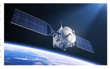
• GSAT-24 is a 24-Ku band communication satellite weighing 4180 kg with Pan-India coverage for meeting DTH application needs.
